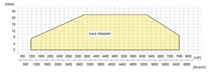
Fig. 1 X = Thermal power Y = Pression in the combustion chamber
