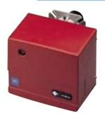
Burners for diesel two stages at two steps of pressure, aluminium frame, protection cover with noise reduction plate, combustion head with micro adjustment at high efficiency and high flame stability, hydraulic system of regulation combustive air on the two stages of flame.
