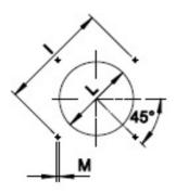
\* Suggested dimension of connection between burner and generator.
