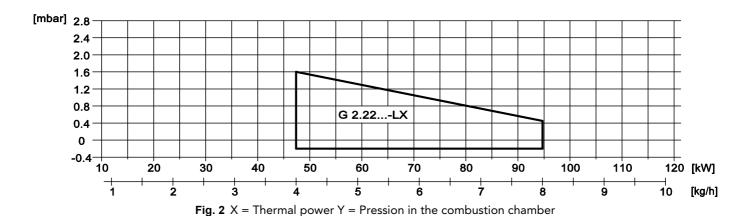
The firing rates has been obtained based on test boilers in accordance with EN267 standards and are indicative of matching the burner to the boiler. For the correct operation of the burner, combustion chamber dimensions must be in accordance with current regulation. In case of non-compliance, contact the manufacturer.
