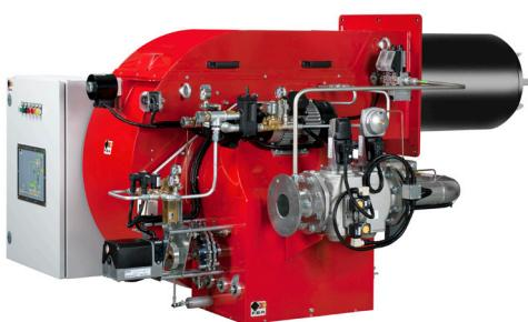
Dual fuel burners for gas and light oil at 2 stages progressive (hi-low flame) or PID fully modulating if optional modulation kit (digital type) and feeder (of temperature or pressure) are added.
