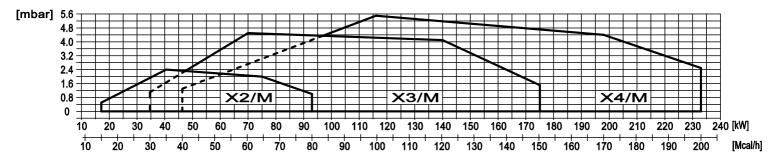
Fig. 4 X = Thermal power Y = Pression in the combustion chamber
