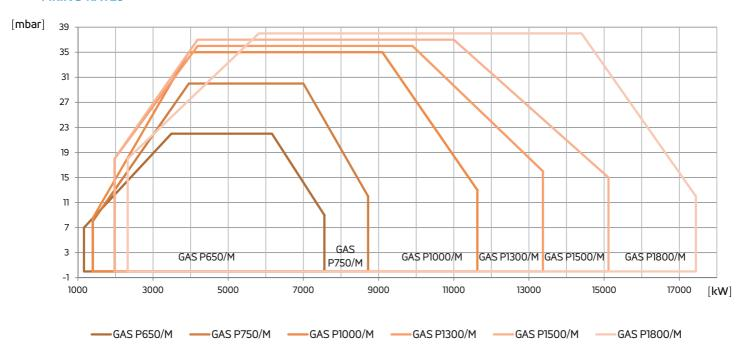
Fig. 2 X = Thermal power [kW] Y = Pression in the combustion
