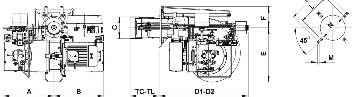
D2= I block to rear burner in maintenance position.
