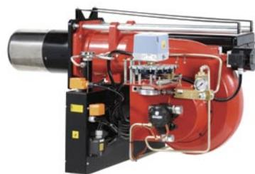
Burners for heavy oil hi/low flame (two stages progressive) or PID fully modulating with the addition of the optional modulation kit (digital) and feeder (of temperature or pressure). Fan at high pressurization , combustion head high efficiency and high flame stability, servomotor for the balanced adjustment of air and oil flow.
