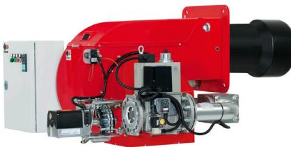
Burners for gas two stages progressive (hi-low flame) or modulating (PID fully modulating) with the addition of the optional system modulation kit plus feeder. Fan at high pressurisation, combustion head with adjustment at high efficiency and high flame stability.
